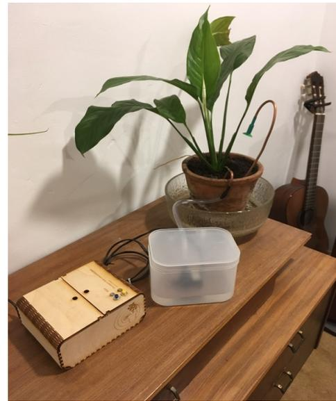
**Figure 1: Plant host installation in the home, showing control box, water reservoir and pump, and waterspout.**
